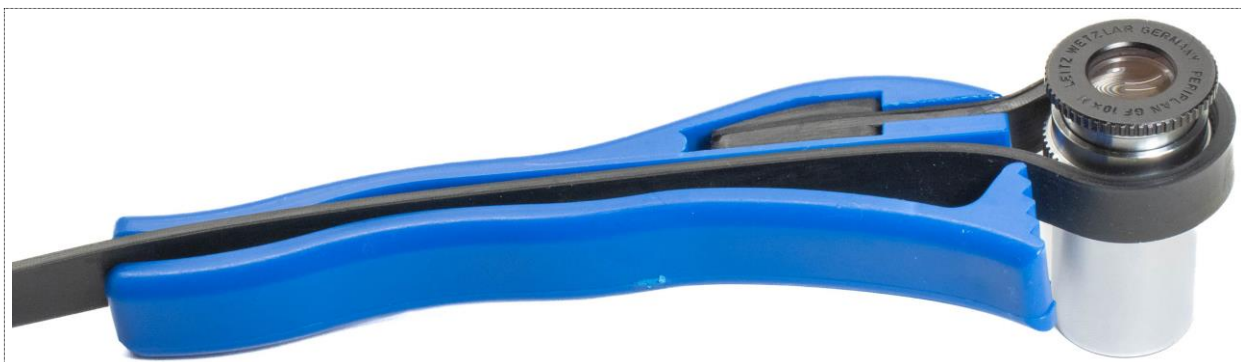
Figure 9: A small strap wrench with the strap tightly wrapped around an eyepiece.
