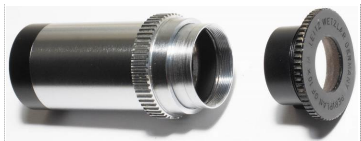
Figure 21: Removal of the eyelens assembly. (The eyepiece in this image is of the “older” eyepiece design.)
