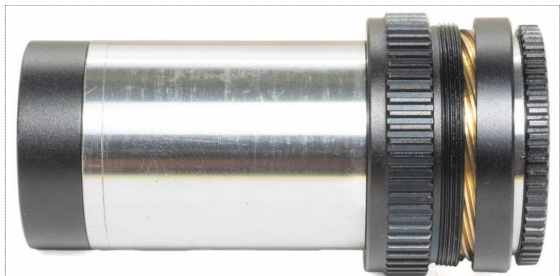
Figure 26: The eyepiece after the locking ring has been released.
