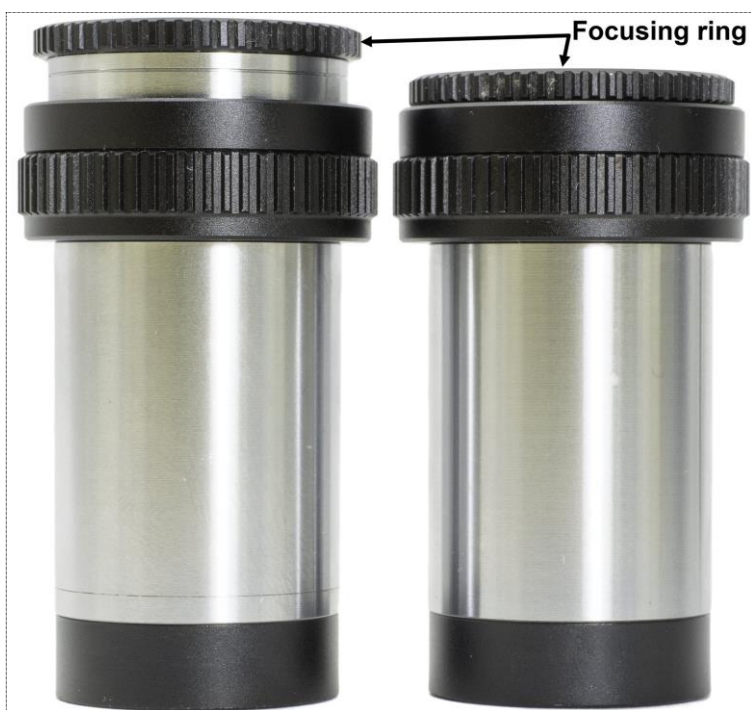
Figure 3: Leitz Periplan GF 12.5x M eyepieces. The focusing eyelens in its most extended (left) and most contracted (right) setting.
