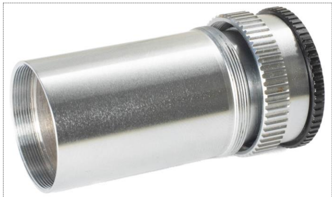
Figure 18: The eyepiece after the locking ring has been released.
