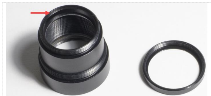
Figure 12: The graticule holder and the graticule holder ring from the field lens assembly. The red arrow points to the circular ledge where the graticule is positioned.
