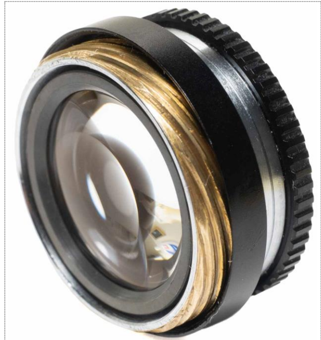
Figure 25: The eyepiece assembly attached to the turning helicoid ring.
